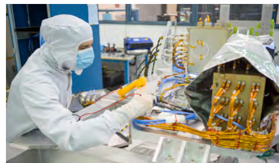
CGI: JPL engineer verifies electrical grounding of avionics systems on the Coronagraph Instrument.
