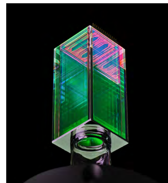
Atomic Chips: Inside this compact vacuum chamber, physicists orchestrate a series of precisely timed cooling stages by applying laser beams, dynamic magnetic fields, and chirped radio waves, culminating in a condensed cloud of quantum gas near absolute zero.
