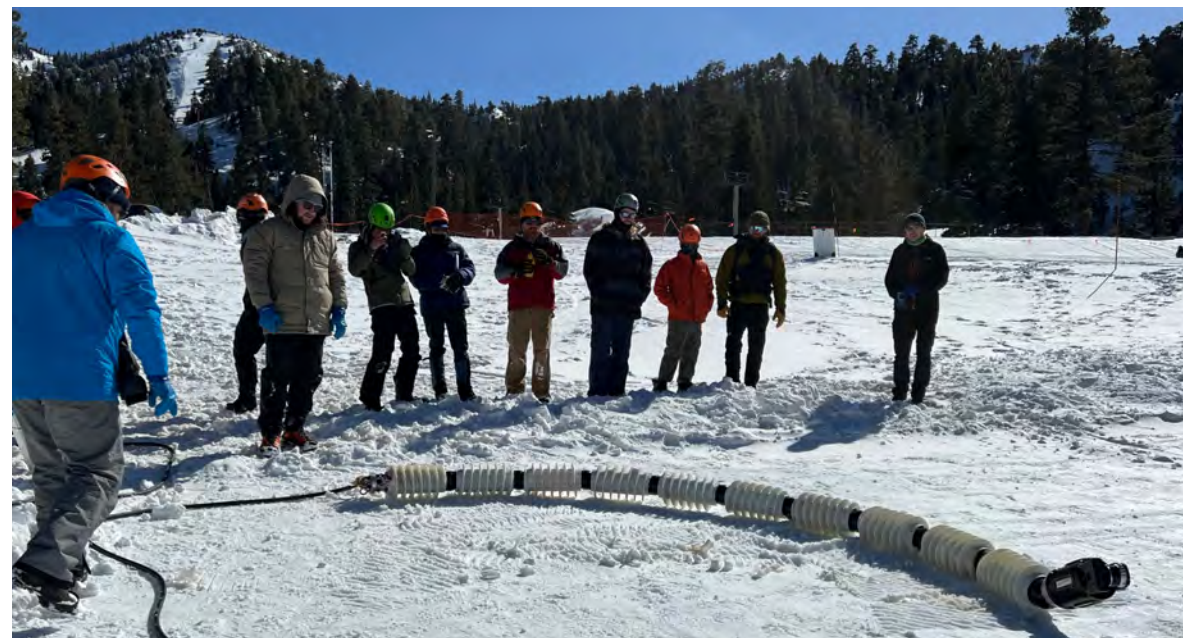
EELS: JPLers test a snake robot called EELS. Designed to sense its environment, calculate risk, travel, and gather data without real-time human input, EELS could eventually explore destinations throughout the solar system.
