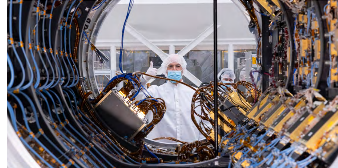
NISAR Assembly: NASA-ISRO Synthetic Aperture Radar being assembled in SAF.
