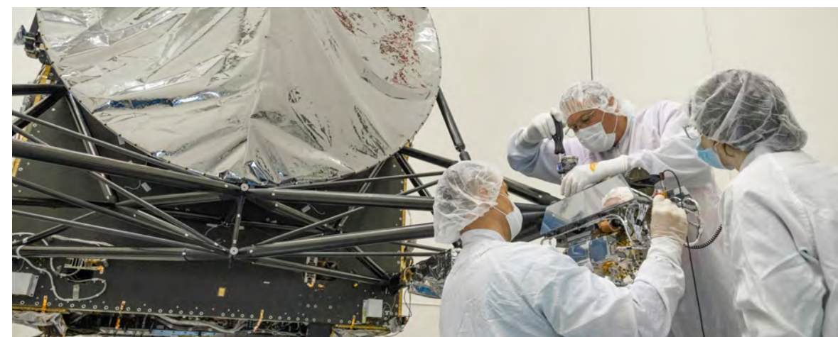
Psyche: Engineers integrate the gamma ray and neutron spectrometer instrument into the agency's Psyche spacecraft.
