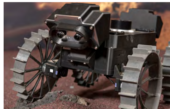
CADRE: NASA's Cooperative Autonomous Distributed Robotic Exploration project is developing a network of shoebox-size mobile robots that could enable future autonomous robotic exploration of the Moon, Mars, and beyond.
