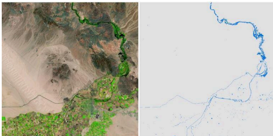
Figure 3.2: Side-by-side images over an area northeast of Yuma, AZ, of a Landsat Surface Reflectance Analysis Ready Data (ARD) tile (left) and a Landsat Level-3 DSWx image (right), reclassified to a binary “water/not water” layer (see Table 3.3). Both images are derived from Landsat 7 ARD Tile Horizontal 005, Vertical 013, collected August 16, 2000. The images are in the public domain and taken from the USGS DSWx site .
