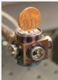
Miniature Microwave Trapped-Ion Clock
