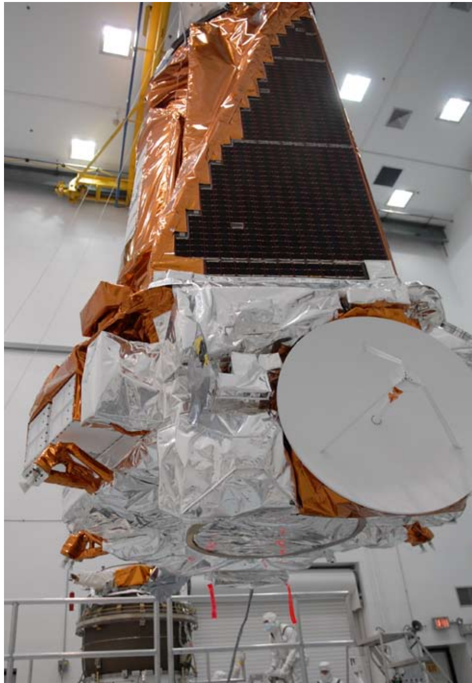
At a processing facility near Kennedy Space Center Feb. 16, the Kepler spacecraft is lifted from a work stand to be joined to a Delta II third stage, in the background.
