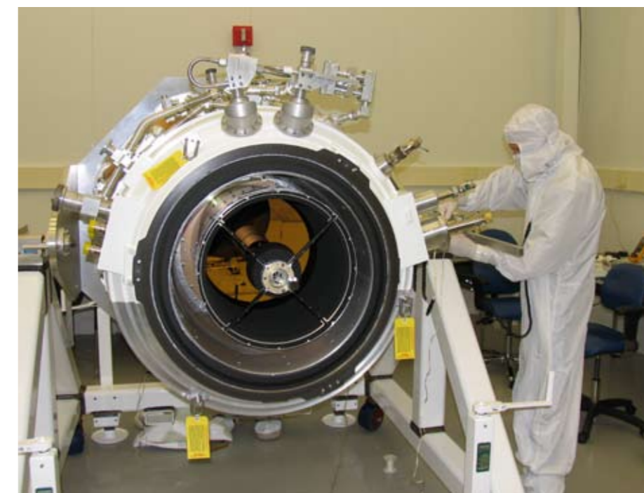
The telescope on the Wide-field Infrared Survey Explorer is shown with the aperture cover removed. The telescope's primary mirror is located at the end of the open tube. This photo was taken during assembly at the Space Dynamics Laboratory in Logan, Utah.
