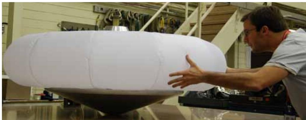
Ian Clark of the EDL Systems and Advanced Technologies Group is shown with a one-fifth-scale model of a candidate inflatable decelerator for the Supersonic Inflatable Aerodynamic Decelerator project.
