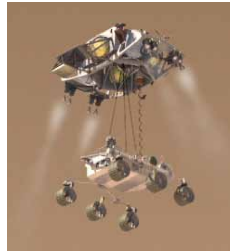
When Curiosity has been slowed to nearly zero velocity, the rover will be released from the descent stage. A bridle and umbilical cord will lower the rover to the ground. The rover's front mobility system will be deployed so that it is essentially ready to rove upon landing.
