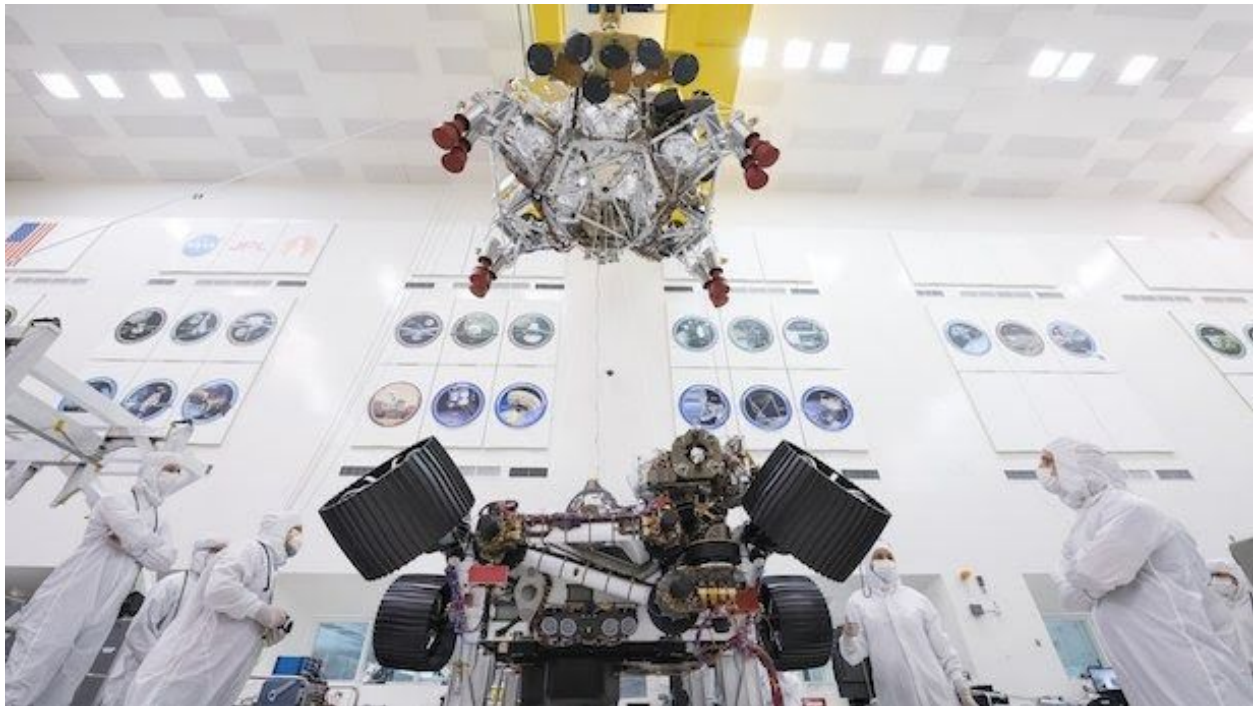
The Mars 2020 rover and descent stage in the Spacecraft Assembly Facility Image Credit: PhotoLab
